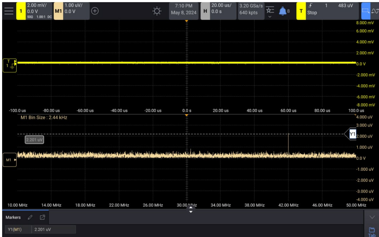
Figure 1. The oscilloscope captures a 2 \mu\text{V} , -100dBm signal very clearly in our FFT. This same signal would not be viewable with a higher noise floor oscilloscope.
